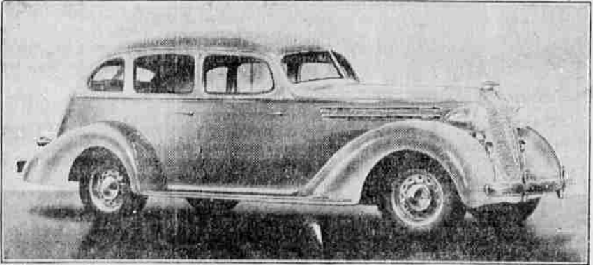
Hudson six-cylinder Sedan. A real six-passenger car mounted on a 120-inch wheelbase chassis. The body is Hudson-built all of steel.
