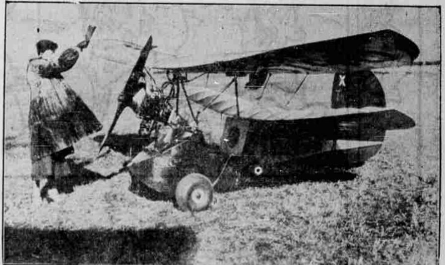
Page Crosley, daughter of Powell Crosley, is pictured as she christened the diminutive plane developed by Edwin Nirmaier, pilot for Crosley. The craft weighs 316 pounds with a wing spread of 19 1/2 feet. (Associated Press Photo)
