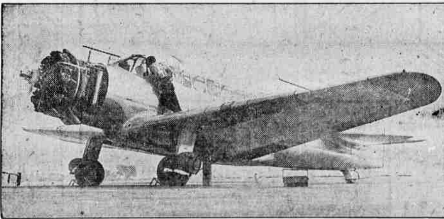
Here is the new Vultee combination bomber and attack plane pictured at the conclusion of the first test flight at Glendale, Calif. It is a sister ship to the one that crashed last month on a test flight killing the two pilots. It was built for a South American government and is armed with five machine guns and carries 1200 pounds of bombs at a 220 mile per hour cruising speed. (Associated Press Photo)
