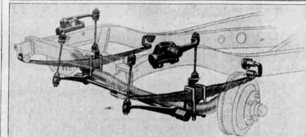
Of intensive interest among the mechanical innovations distinguishing the 1935 Dodge models is the new-front suspension. The system incorporates a rigid front axle, double-acting hydraulic shock absorbers, leaf springs of twice the usual softness, and a ride "levelator"
