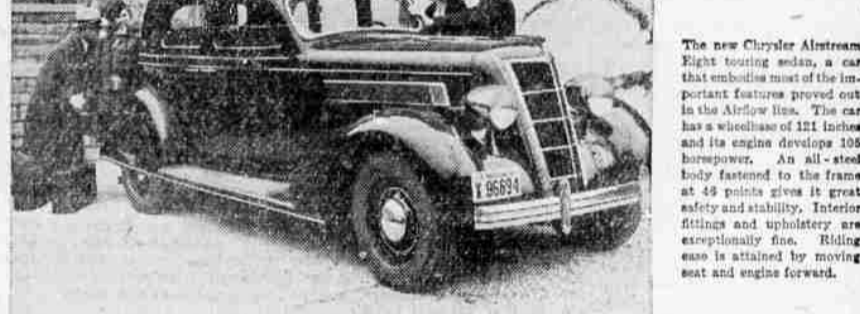
The new Chrysler Airstream Eight touring sedan, a car that embodies most of the important features proved out in the Airflow line. The car has a wheelbase of 121 inches and its engine develops 105 horsepower. An all-steel body fastened to the frame at 48 points gives it great safety and stability. Interior fittings and upholstery are exceptionally fine. Riding ease is attained by moving seat and engine forward.
