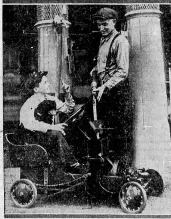
Associated Press Photo Stanley McCrary is telling the service station attendant to "fill 'er up," which means one gallon. His little automobile, made of odds and ends, is propelled by an old washing machine motor. High speed is 12 miles an hour and fuel consumption "about a gallon of gasoline a day." Stanley says it's a great improvement on scooters and such.
