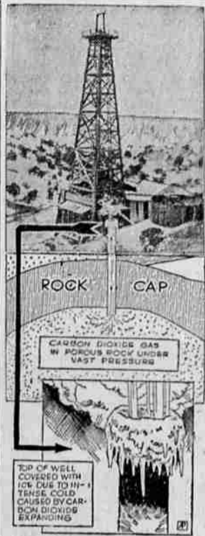
Diagram shows how carbon dioxide gas from 3,000 feet underground in Utah forms commercial "ice" as it expands when released from underground pressure at the mouth of the well.
