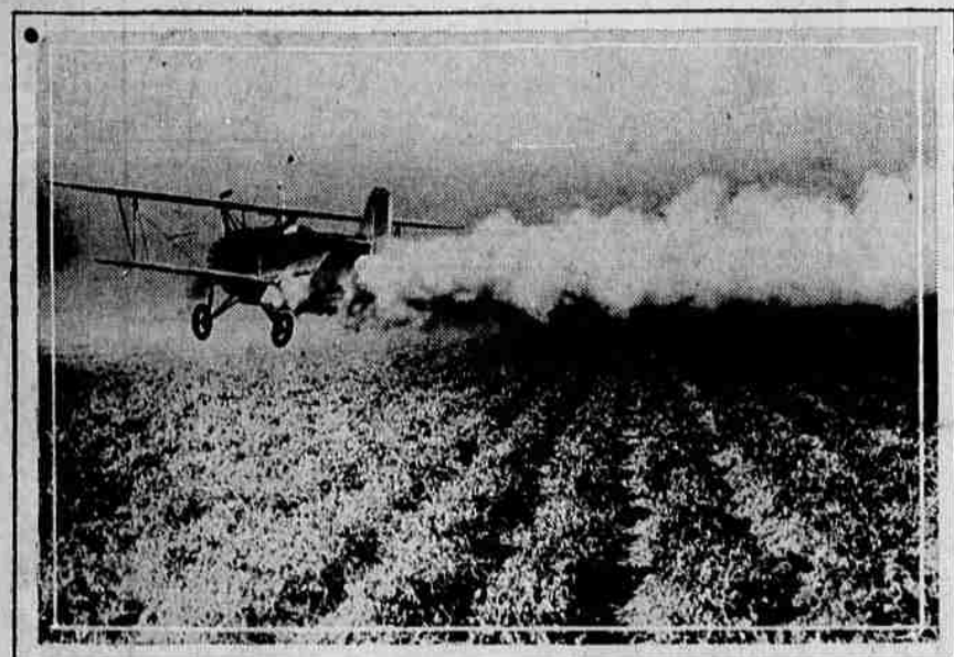
THIS SPECTACULAR PHOTOGRAPH shows how 1,000,000 acres of land in New Mexico are being disinfected by low-flying airplanes to remove plant parasites. A specially devised plant-dusting machine, pictured in action above, carries insecticide aloft by the ton and blows it over the large area quickly and effectually.
