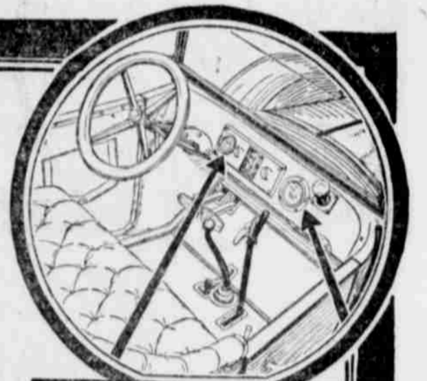
Speedometer, fuse box, ignition, lights, battery regulator, all mounted flush on instrument board.
