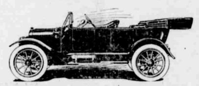
Four-cylinder, 25-horsepower motor, cone clutch, three-speed transmission, unit power plant, 3-4 floating rear axle, five-passenger, Prestolite tank, nickel trimmed, 103-inch wheel base, 30x31/2 tires all around.
