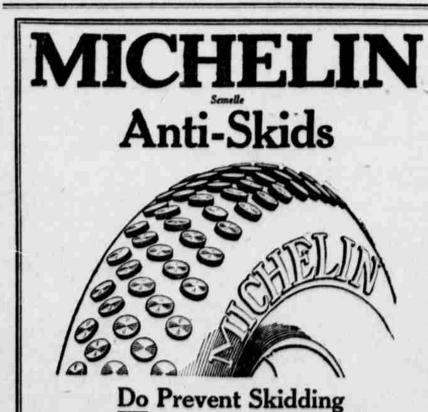
Rubber Traction Surface Protected and Reinforced by Tough, Flexible, Non-puncturing Leather Tread, An In-tegral Part of the Tire and Not An Attachment. Firmly Imbedded Hardened Steel Studs Do Prevent Skidding.
