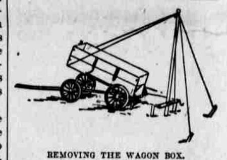
REMOVING THE WAGON BOX.
