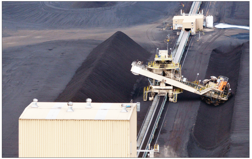
A stacker reclaimer digs up scoops of coal to feed a conveyer belt that fuels the Boardman Coal Plant.
