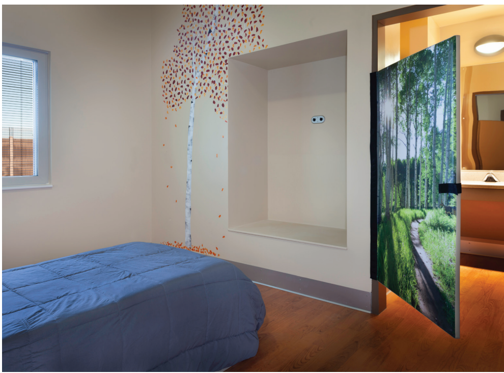
The 16 private patient rooms feature attached bathrooms with flexible mat doors that provide privacy without allowing people to barricade themselves inside.
