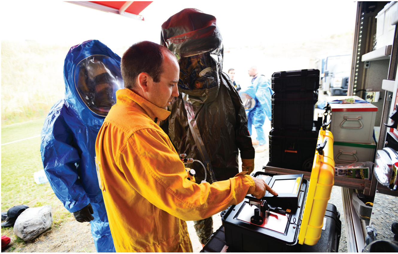
Lt. Matt Fisher, center, demonstrates how to use a HazMat 360 infrared spectroscopy to firefighter Matt Lewis, left, and Lt. Jeff Armstrong on Thursday while training in Hermiston. The infrared spectroscopy, which uses a laser to determine chemical compounds, is a valuable tool for firefighters responding to hazardous materials incidents.
