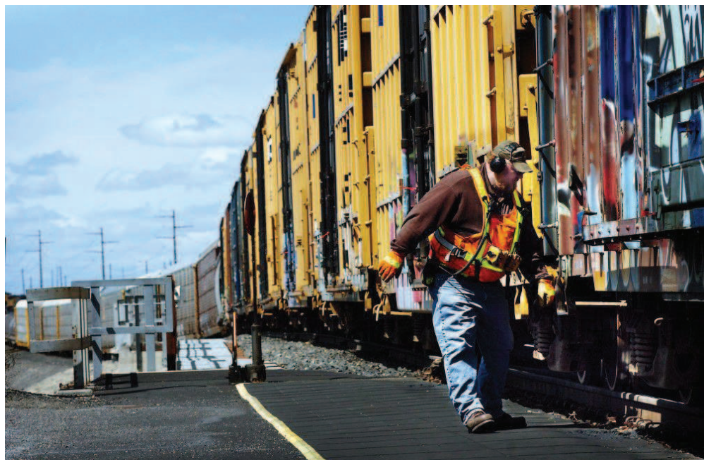
A remote control operator decouples a rail car in July 2012 while taking apart a train at the Union Pacific Railroad Hinkle Locomotive Service and Repair Facility and Freight Classification Yard near Stanfield.
