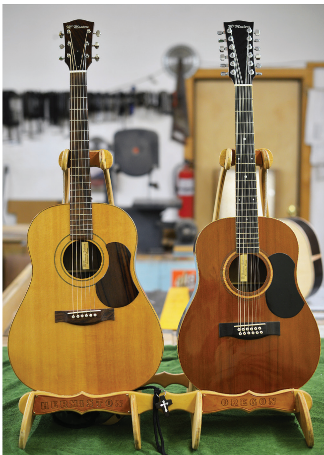
Guitar maker Les McMasters likes to use a wide variety of woods in the creation of his guitars. The instrument on the left is a Gibson jumbo styles Guitar with Bolivian rosewood on the back and Sitka spruce on the top. The guitar on the right is a twelve-string lady's fancy guitar in what McMasters has dubbed his "Oregon guitar" with a Redwood top from southern Oregon and a back using black walnut from Baker City.
