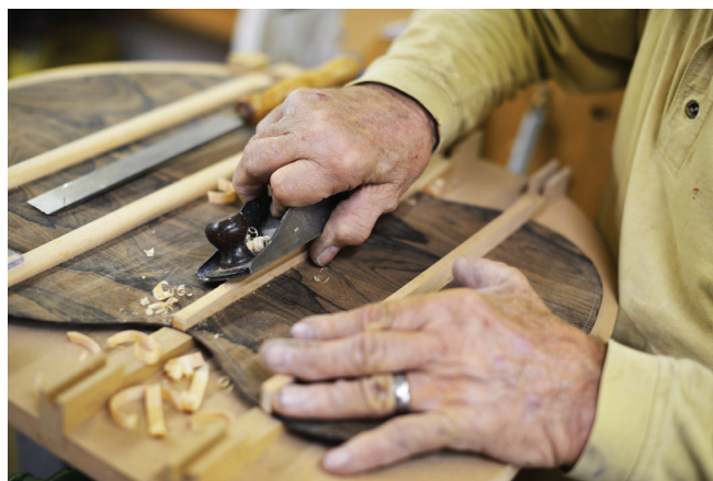
Les McMasters uses a block plainer to shape the braces on the back of a guitar at his shop in Hermiston.
