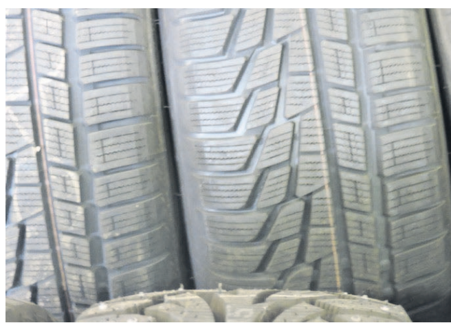
Studded (foreground) and studless snow tires sit side by side at G&S tire Factory in Hermiston. Note the similarities in siping of the two tire types, yet the absence of studs on the tires in the back.
