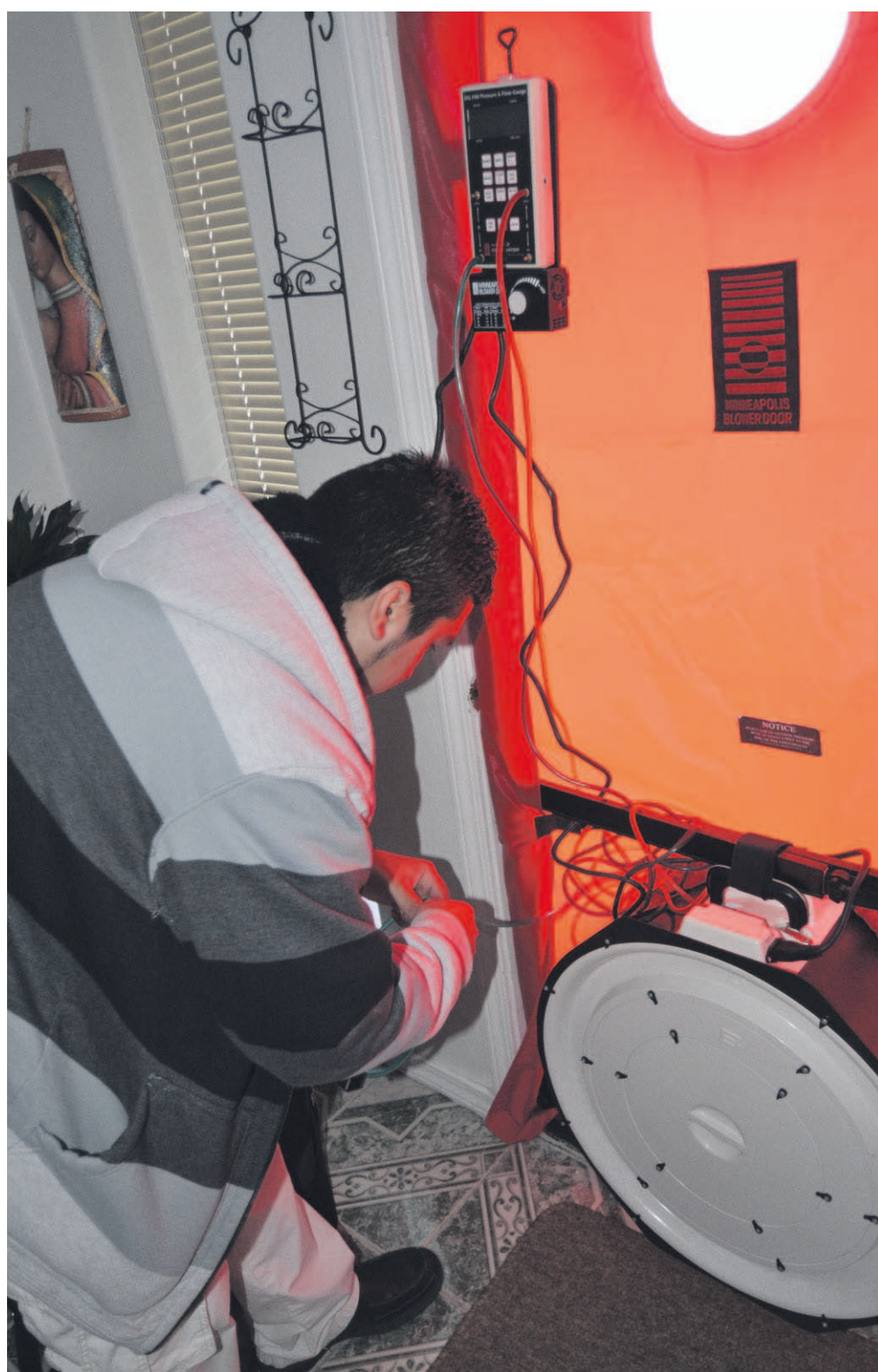
PHOTO COURTESY UMATILLA ELECTRIC COOPERATIVE Gerardo Villegas of Umatilla Electric Cooperative prepared to conduct a blower door test as part of an energy audit to determine where drafts may exist in a home.
