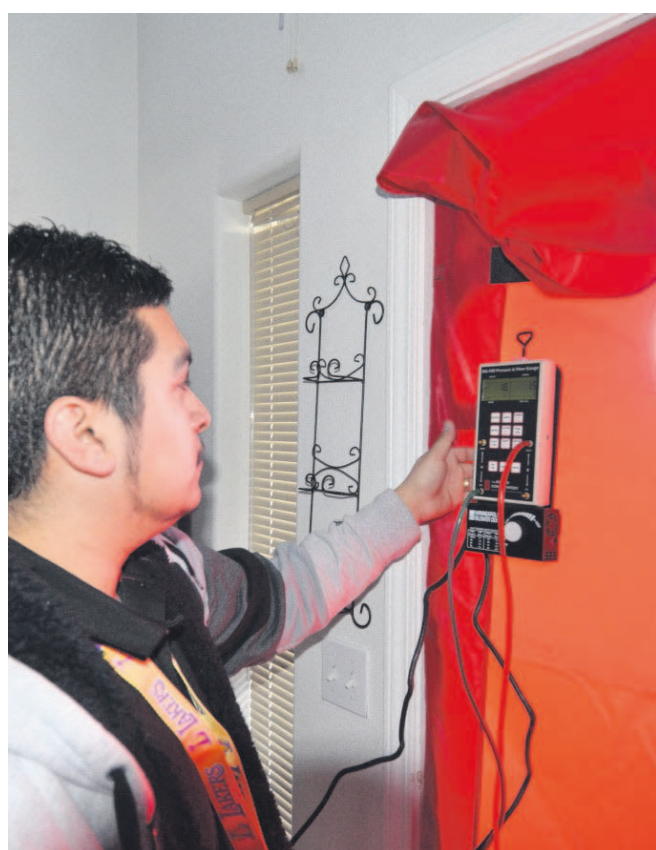
PHOTO COURTESY UMATILLA ELECTRIC COOPERATIVE Gerardo Villegas, efficiency representative for Umatilla Electric Cooperative, sets up blower door test equipment during an energy audit.
