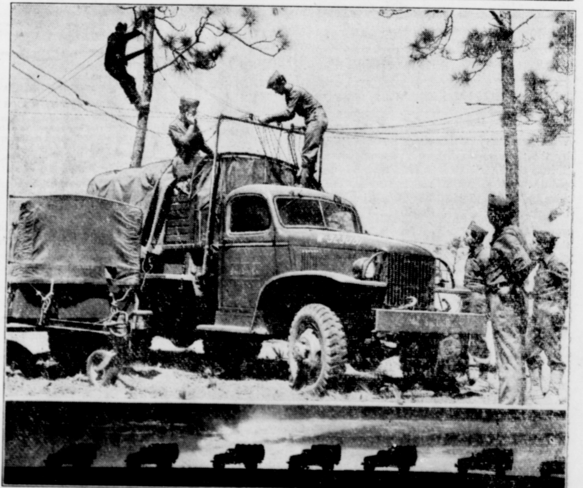
Uncle Sam's motorized force—the new army on wheels—is symbolized by the "dawn patrol" of Chevrolet 4 x 4 army trucks shown across the bottom of the photo. The Chevrolet four-wheel-drive army truck, above, carries a complete telephone switchboard. Within a few minutes after the Fourth Division's motorized units completed a 235-mile trek from Fort Benning, Ga., on a practice maneuver, Major-General Lloyd R. Fredendall could communicate with every part of the vast encampment. The Fourth, moving in three columns, each 45 miles long, made the trip in 10 hours as compared with nearly 10 days before motorization.
