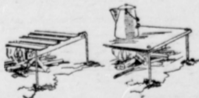
Camp-Stove Top, Either Solid or Pierced, Supported on Rods at the Corners.
