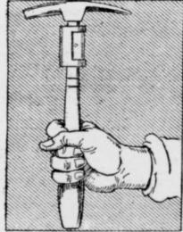
cently been invented which is always to be found with the tacks. Just under the head of the tool there is secured to the handle a circular magazine arrangement for holding tacks. This has a sliding door by which the contents may be exposed, and when it is desired to close it there is an automatic catch which holds it in place.
