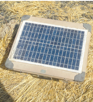
Solar power cell used to charge mobile electric fence. -Continued from PAGE ONE
