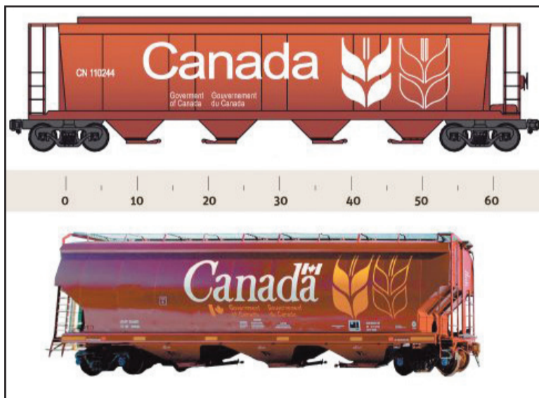
This is a similar graphic pointing out the difference between a standard capacity train hopper and the new train hopper used at the POM. - Contributed Photo
