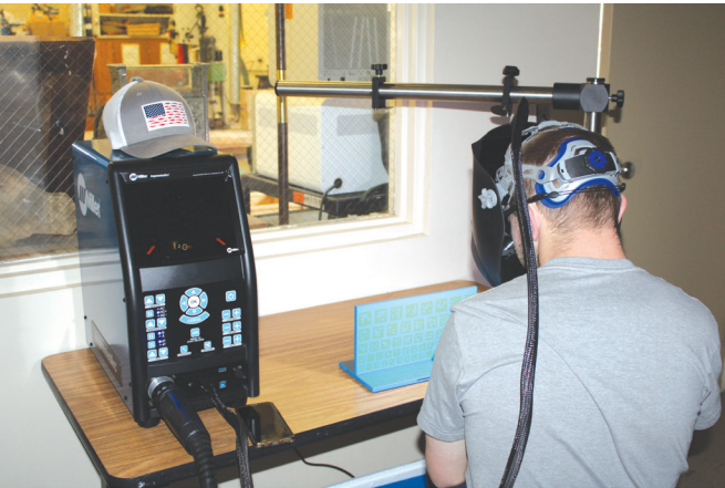
Ione senior Calvin Rietmann works with the school's new augmented reality welder, which allows students to practice welding through a combination of real objects and virtual reality. -Photo by Andrea Di Salvo
