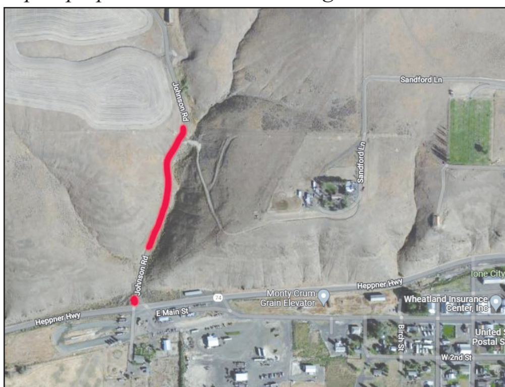
Ione's proposed new sewer system to pump effluent up Johnson Grade to large drain field
