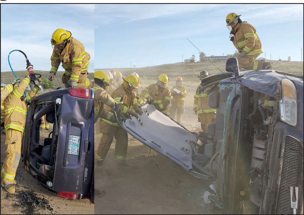
The three local fire departments of Heppner, Lexington and Ione got some training and practice last week using the rescue tool Jaws of Life. The tool is used to cut away parts of vehicles for quicker rescue of crash victims. The firemen first cut the stanchions and then completely remove the top of a practice car. Not only do the firemen get practice but they also are recertified on using the tool, says Fire Chief Steve Rhea. In addition to training on a car with the tool the firemen also receive two 2-hour classes on its use. Martin Towing of Lexington provided three vehicles for the firemen to practice on. History of the jaws tool goes back to 1961 when George Hurst invented the Hurst Rescue Tool after he viewed a stock car race accident in which it took workers over an hour to remove an injured driver from his car. The tool was a great improvement over saws and crow bars also used in rescue. -Photo by David Sykes.
