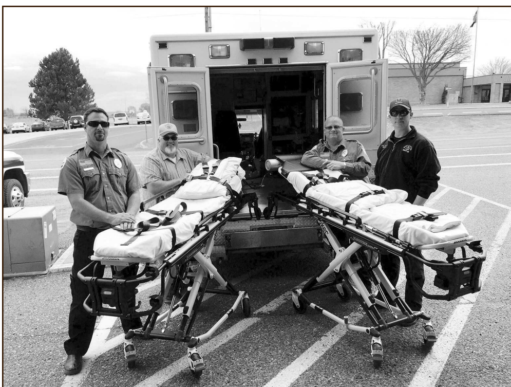
Morrow County Health District has purchased new Stryker gurneys for every ambulance in Morrow County, reports Emergency Medical Services Coordinator Rusty Estes. The new gurneys are hydraulic with a 700-pound lift capacity. Estes says the purchase will make ambulance transports safer both for patients and the EMTs loading them onto the ambulance; medics and drivers say they are excited to have the new gurneys. The purchase was made possible by funding from CREZ (Columbia River Enterprise Zone), Wildhorse Foundation, and the MCHD Board. Pictured (L-R): Boardman paramedic Devon Pulvino, EMS Coordinator Rusty Estes, Boardman paramedic Del Turner and Irrigon paramedic Kelly Shelton. -Contributed photo
