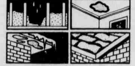
3. AUTOMATIC ATTIC VENTILATION protects against winter moisture damage to insulation ceilings, paint, roof boards and shingles.
