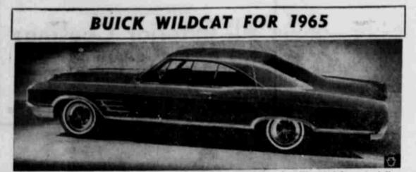
The semi-fastback styling of two-door models in Buick's 1965 line is epitomized in the Wildcat with its longer hood, lower, longer rooflines and short rear deck. Three inches have been added to the hood by increasing the wheelbase from 123 to 126 inches for improved riding and handling. Overall length remains approximately the same as last year. A new cross-flow radiator design permits lowering the hood line on all models in LeSabre, Wildart and gear box are optional on the Wildeat.
