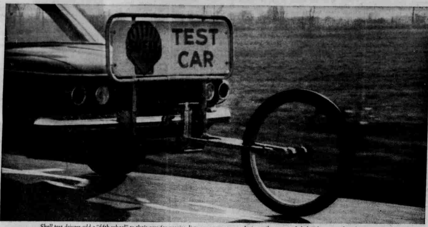
Shell test drivers add a "fifth wheel" to their cars for precise distance measurement during mileage tests. It helps them record performance to a decimal point.
