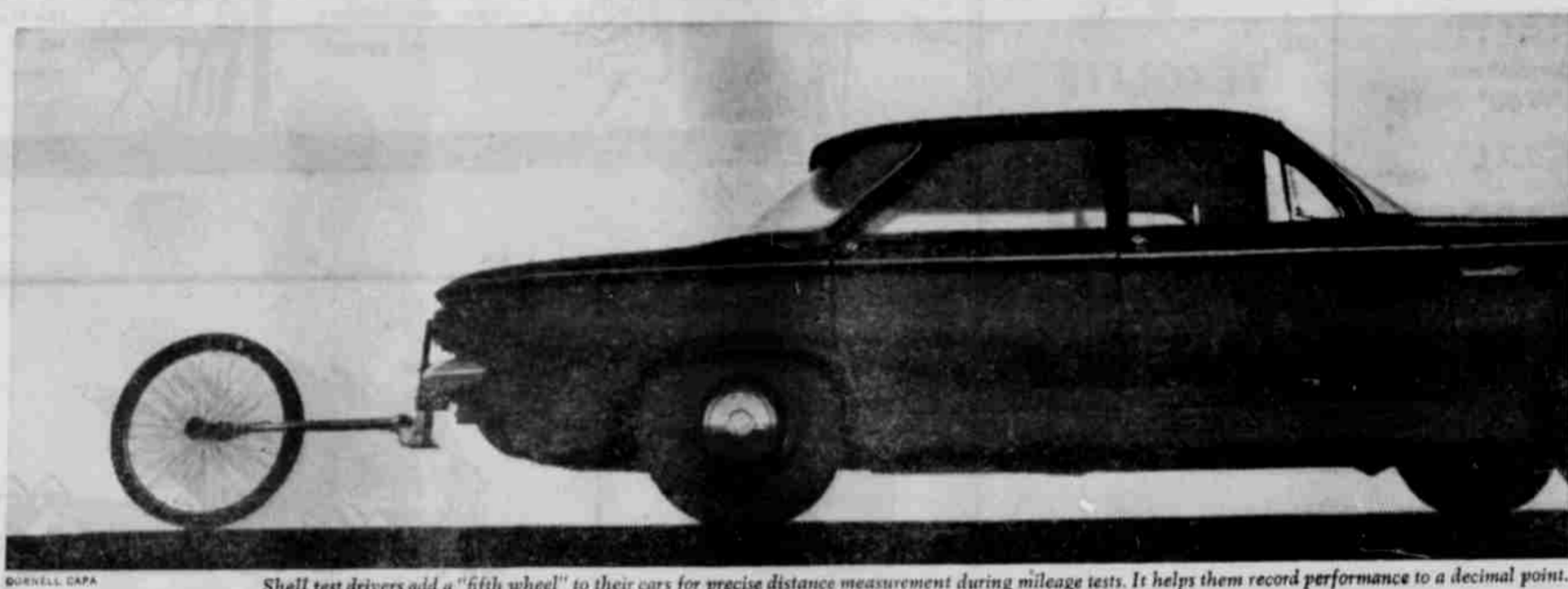
Shell test drivers add a "fifth wheel" to their cars for precise distance measurement during mileage tests. It helps them record performance to a decimal point.
