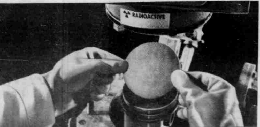
These gloved hands are placing a piece of sensitized film on a radioactive piston. This produces what is known as a "radio autograph," from which Shell's scientists can study the nature of deposits.
