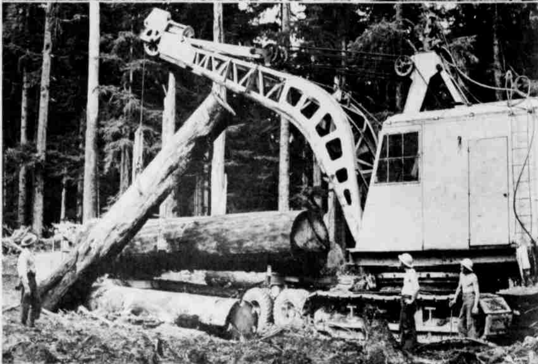
EARLY DAY LOGGING operations centered around the steam-powered "Giffert" log loader. Empty cars were backed under the loader and moved forward as each load was completed. No railroad is needed for the modern loader, for its tracks transport the heavy equipment where it is needed and the logging truck backs up to the loader to receive its logs.
