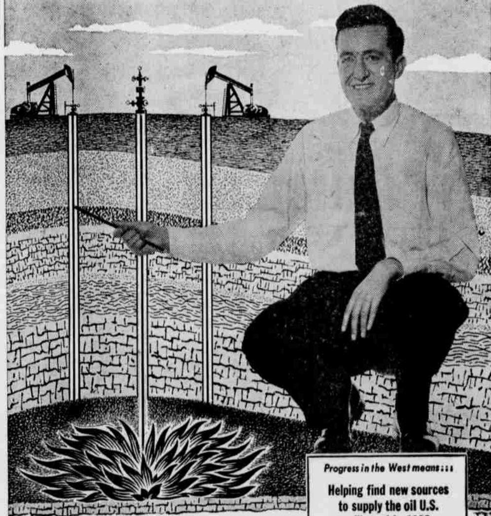
Fire flooding produces heat and pressure to boil out previously unrecoverable oil, driving it underground to nearby producing wells.
