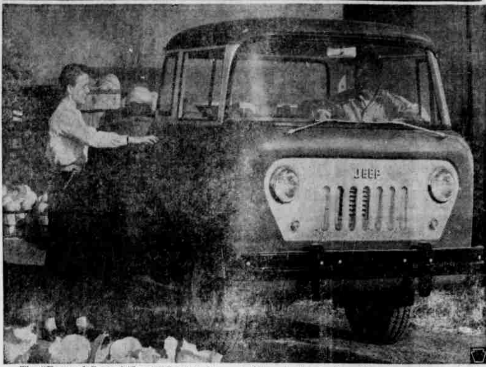
The "Forward Control Jeep" FC-150, all-new addition to the expanding line of Willys Motors four-wheel drive vehicles, is now being introduced by Willys dealers. Key feature of the new model is the "up-front" location of the cab, which allows maximum usage of the vehicle's compact wheel-base for payloads, and at the same time places the driver in the best position for split-second all-direction visibility. The FC-150 is powered by the same F-head "Hurricane" engine proved for ruggedness and economy in the "Jeep," and is engineered with four-wheel drive for off-the-road service over all types of terrain.
