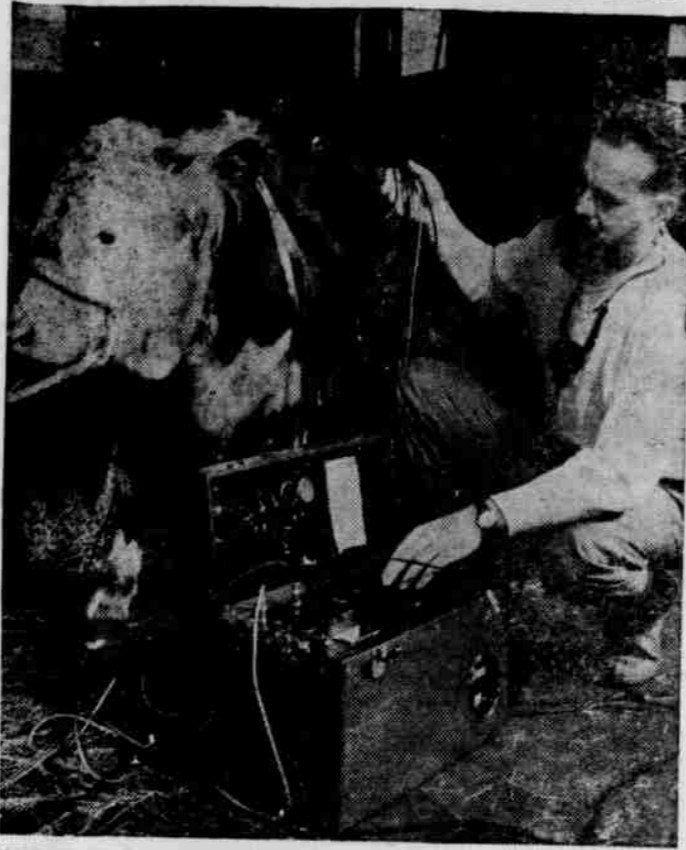
THE ELECTROCARDIOGRAPH, same instrument which doctors use to study the human heart, is being used by Oregon State college scientists in studies of white muscle disease in cattle and sheep. The disease, which affects the heart, causes serious loss of calves and sheep in Oregon. Electrical activity of the heart is recorded to show visually the condition of the heart. OSC scientists are determining standards for normal and abnormal beef hearts. Studies are part of a program to learn more about adjustments of cattle under various environmental conditions with the aim of improving beef production. William Van Ardel (above) is a graduate student at OSC.
