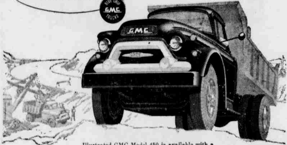
Illustrated GMC Model 450 is available with a 180 h.p. V8 engine or 160 h.p. six. It has over-size axles—7,000 lbs. front and 18,000 lbs. rear. It's rated for 25,000 GVW-50,000 GCW work.
