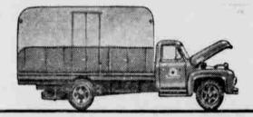
NOW 1/4 TON MORE GVW-Ford Series F-750 now has GVW upped to 21,000 lbs. when equipped with heavy-duty rear springs. 152-h.p. Short Stroke V-8 engine. Power Steering available.
