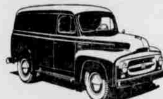
PANELS: R-110 Series. 115-inch wheelbase. Loadspace dimensions, length 90 inches, width 60 inches, height 54 inches. Rear doors open to 90° or 180° positions. Overdrive optional.
