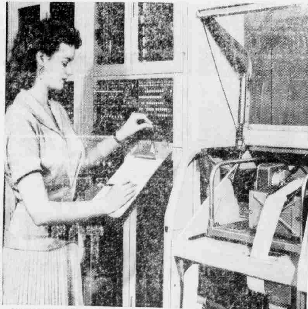
This automatic recording machine keeps track of your calls on tape, permits you to dial farther.
