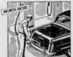
Center-Fill Fueling prevents hose marks on the finish of your car. No gas spill on fenders. Short gas filler pipe gives you trunk space for an extra suitcase.
