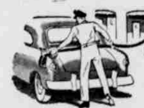
THE OLD WAY—Gas filler cap on fender... unhandy to reach from far side... unsightly.
