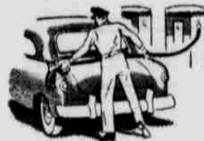
THE OLD WAY—Gas filler cap on fender...unhandy to reach from far side...unsightly.
