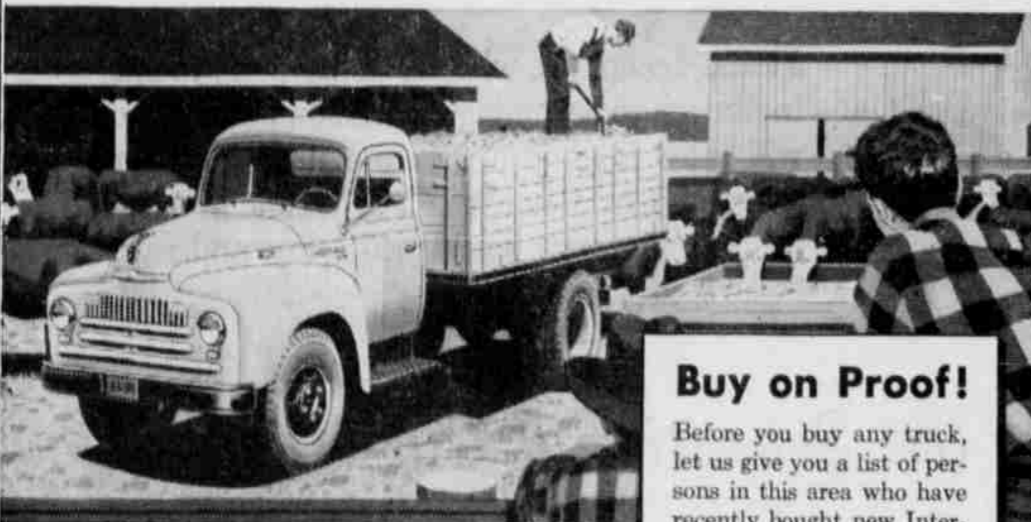
International L-160 models offer 130 to 172-in. wheelbases, GVW ratings from 14,000 to 16,500 lbs.
