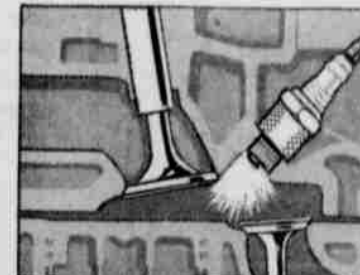
Free-Breathing F-head design and 7.6 compression give more power and mileage from every drop of gas in the Hurricane 6 Engine.
