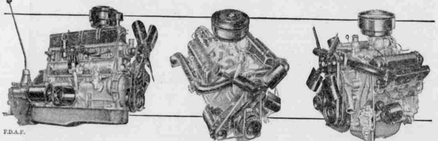
101-H.P. COST CLIPPER SIX: New LOW-FRICTION design, 212 cu. in. Available Series F-1 thru F-3.
