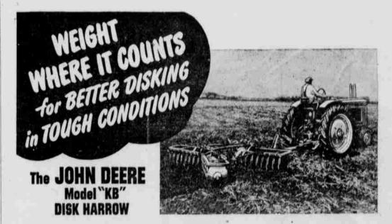
Hard-baked stubble, stubborn stalks, and heavy trash meet their master when you enter the field with a John Deere "KB" Heavy-Duty Disk Harrow. The husky Model "KB" makes short work of the toughest disking jobs because proper weight distribution of the heavy-duty frame holds the gangs to their work and assures good, uniform penetration.
