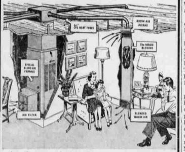
Above, the furnace is located in the utility room with heat tubes in the attic. With basement installation, heat tubes are beneath floor.
