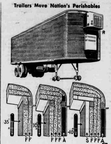
The nation's perishable food supply is moving over the highway in mechanically stainless steel refrigerated trailers. As a result farm products are reaching America's tables fresher and more palatable. Food products are transported at proper temperatures. Frozen foods, for example, have to be kept as low as 10 degrees below zero, say Fruehauf Trailer company engineers.
