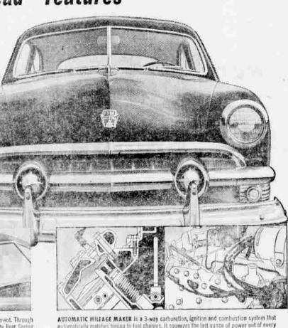
automatically matches timing to fuel charges. It squeezes the last ounce of power out of every drop of gas..., gives you high compression performance with regular gas. And Ford's new Waterproof Ignition System delivers quick starts in the wettest weather
